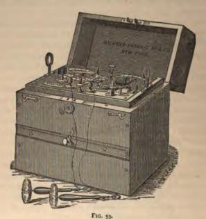
Twenty-four-cell zinc-carbon battery with hydrostat.
